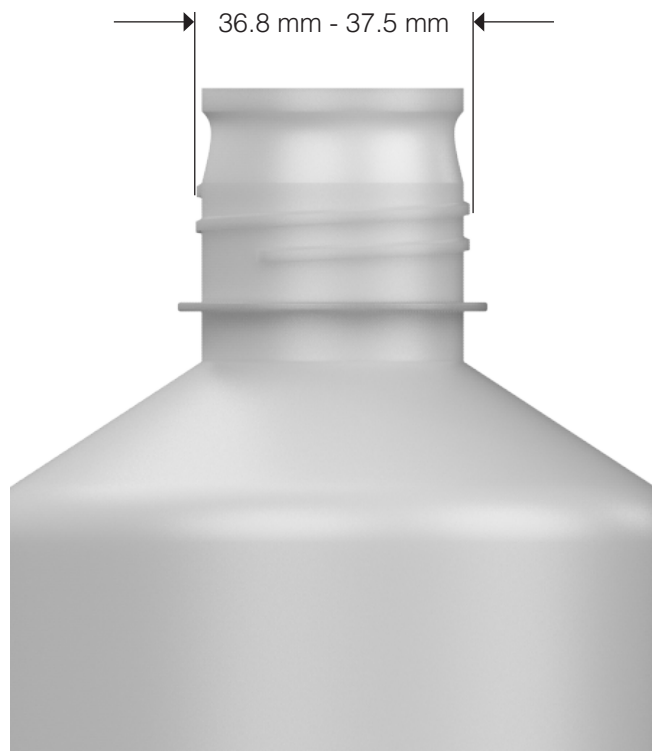
38-430 plastic thread (Nalgene and similar) Scale 1:1
