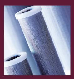
MicraMesh Stainless Steel filter cartridges are manufactured from five layers of mesh sintered together to form an integrated porous filter cartridge. This type of cartridge retains solid and liquid contaminants from gas samples and solid contaminants from liquid samples. These filter cartridges also offer excellent corrosion and pressure dierential resistance and are supplied complete with a fitted PTFE gasket. MicraMesh filter cartridges are suitable for use with MicraSteel filters.
