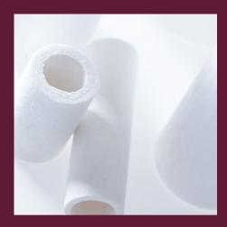
MicraLescer are high effciency, self-supporting, fluorocarbon resin bonded, borosilicate glass microbre filter cartridges. Suitable for use in gas and liquid applications, the MicraLescer cartridges are designed to coalesce liquid particles through a two layer construction. The inner layer forms the main filtration and the coarser outer layer provides drainage. Typical applications include two phase separation i.e. oil aerosol from air (or gas), oil from water and water from oil.
