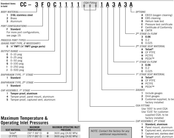
3600 psig (24.82 MPa) CF PTFE 175° F (80° C) 3600 psig (24.82 MPa) PEEK™ 175° F (80° C) @ **PCTFE** 175° F (80° C) 3600 psig (24.82 MPa)
