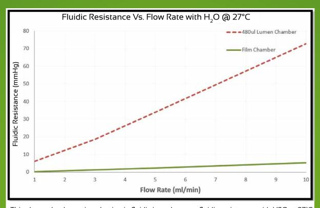
This shows the dramatic reduction in fluidic impedance, or fluidic resistance, with H2O at 27°C. There is ~0.1 PSI of resistance from 1 to 10 mL/min. This is about 5 mmHg pressure drop over the flow rate range.
