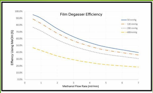
A characterization of the new flat film degasser at various vacuum levels and flow rates produces a data set from which any particular performance curve can be derived. This data set allows complete control over the efficiency of the degasser, such that the degasser can be optimized for any flow rate within the vacuum range of the pump.
