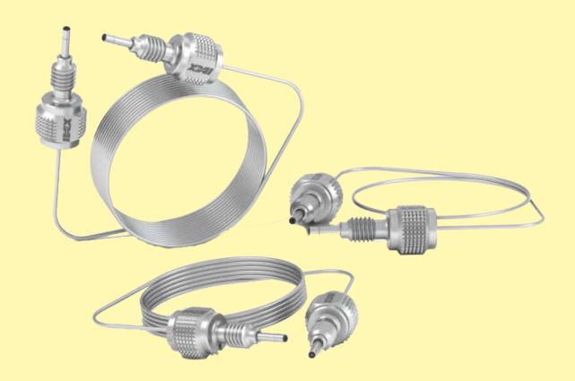
The BioVersal<sup>™</sup> sample loops are 100% bioinert, making them ideal when injecting biological or "sticky" samples. The PEEK lining reinforced by the stainless steel gives these sample loops the strength to withstand pressures up to 1310 bar (131 MPa; 19,000 psi), and makes the sample loop inert to almost all organic solvents.
