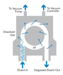
Dissolved gases are actively removed from a flowing liquid stream by vacuum via the IDEX Health & Science AF® membrane.
