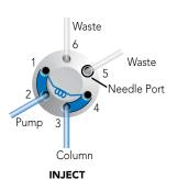
analysis, and/or you have an abundance of sample, either a dual mode or single mode injector is appropriate. Both types of injection valves allow the complete-filling method in which you overfill the sample loop. Complete-filling maximizes the reproducibility of your results.
