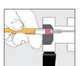
**Figure 1** To reform the needle seal, push the eraser end of a pencil against the needle port
