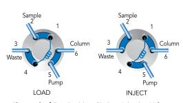
Flow path of Two-Position, Six-Port Injection Valve
