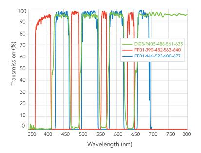
BrightLine multi-band N2 flatness super-resolution laser filter set, optimized for 405, 488, 561, and 635 nm laser sources.
