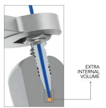
MarvelX UHPLC fittings do not depend on ferrules. They seal at the bottom of the port, without complex techniques, which significantly reduces required torque and enables many more connects and disconnects. Furthermore, they are virtually impossible to over-tighten by hand, limiting wear and increasing product life. An enhanced proprietary tip design also ensures zero dead volume (ZDV) and better chromatography results.
