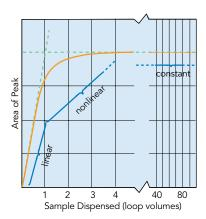
Figure 2 Sample mass (observed peak area) vs. volume of sample dispensed from the syringe, in units of loop volumes, injected onto the column from our dual mode injector such
