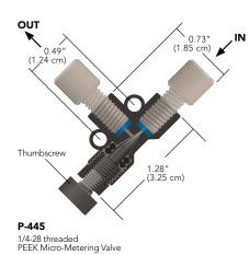
For fine control of fluid flow rates, Micro-Metering Valves can reduce outgoing flow to as low as  $3.5 \,\mu$ L/min\*. These needle valves are perfect for use with peristaltic pump fluid-transfer applications, mass spectrometry, and fraction collection.
