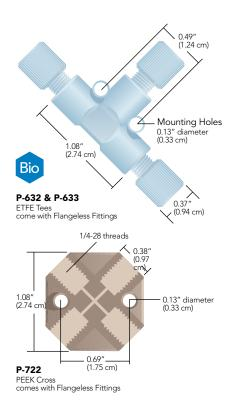
Our Low Pressure Tees and Crosses are available in two inert polymers and can handle pressures to 500 psi (34 bar) or 1,000 psi (69 bar), depending upon the configuration of the products. Each is designed with handy mounting holes. All ETFE Tees and Crosses ship complete with 1/4-28 PFA Flangeless nuts and ETFE ferrules, while their PEEK polymer counterparts ship with 1/4-28 PEEK nuts and ETFE ferrules. Replacement fittings are located on page 47.
