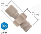
1/8" NPT to 5/16-24 Flat-Bottom Female Adapter for 3/16" OD tubing Includes (1) XP-132 Fitting
