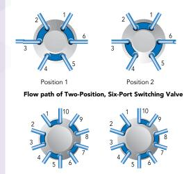
Flow path of Two-Position, Ten-Port Switching Valve
