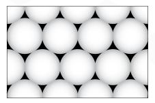
Frit volume is calculated by determining what the mass of the frit would be if it were a solid block of material of equal size. Then the solid mass of the frit is multiplied by the percentage assigned to the porosity to determine the theoretical frit volume.
