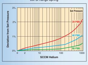
The Porter Model 9000 Regulator is a compact, spring-loaded, diaphragm operated back pressure regulator. Designed specifically for precision regulation in low-flow gas applications, it controls upstream pressure rather than downstream pressure and is similar to a relief valve in operation.
