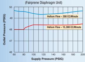
The Porter Model 8286 Regulator utilizes a pneumatically balanced poppet valve to ensure maximum stability over wide variations in supply pressure. It is direct acting, non-relieving, and is supplied with a replaceable sintered stainless steel cartridge filter on the inlet. It can be equipped with a stainless diaphragm for reduced permeability. The Model 8286 is performance tested under simulated operating conditions and is cleaned for analytical instrument service.
