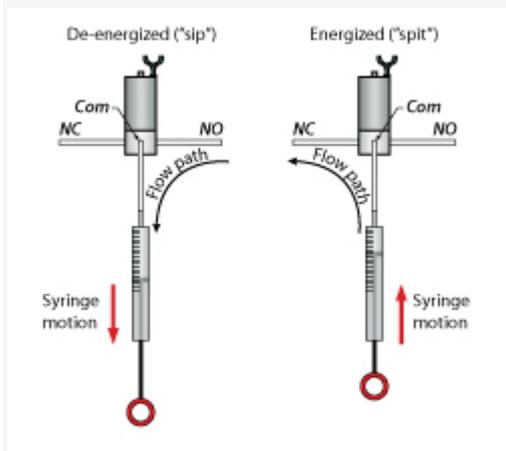
Sometimes the volume of liquid to be dispensed needs to be either very small, extremely precise or both. In these situations, it is very common to use a precision machined syringe to control the dispense volume.
