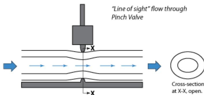
Pinch Valves offer "line-of-sight" flow paths where the open tube, even if slightly pinched does not significantly block the flow
