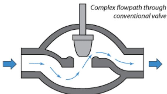
Conventional on-off valves often require the fluid to be regulated to move through a convoluted / complex flow path, even when fully open. This can be an issue for biological materials (proteins, DNA, etc.) which can be easily "sheared" when forced through complicated paths.
